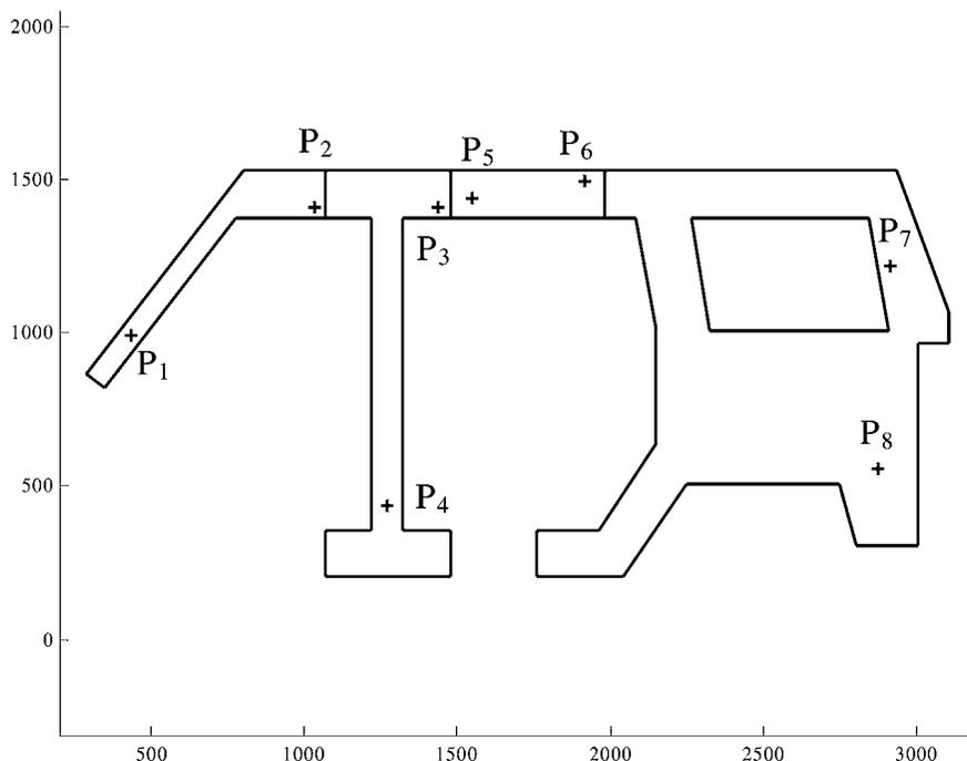
Figure 7. Optimal Fixture Layouts With the Lowest  $S$  Value.
