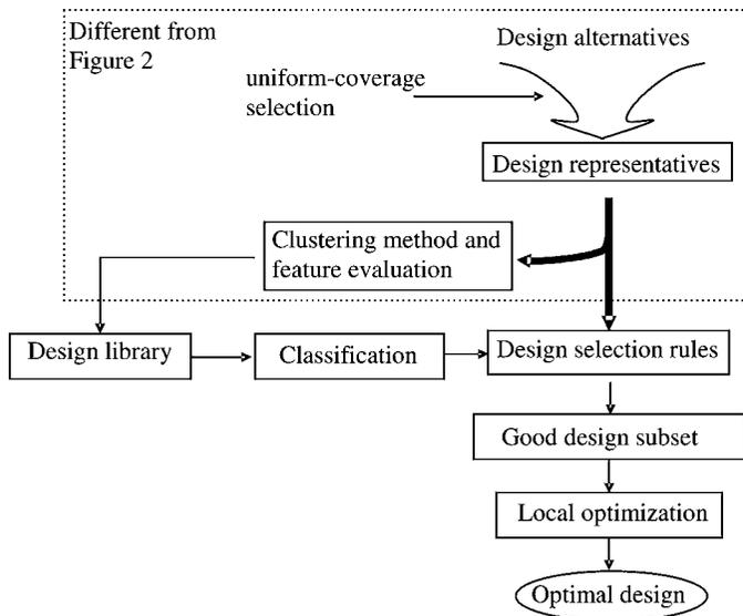
Figure 3. Modified Data-Mining-Aided Design Optimization Procedure.
