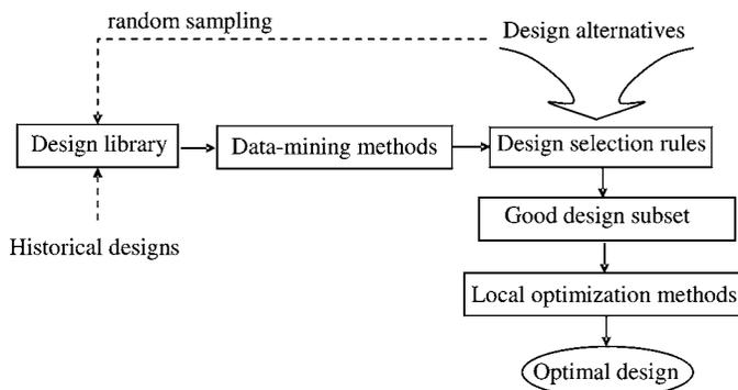
Figure 2. Design Optimization Using Data-Mining Methods.
