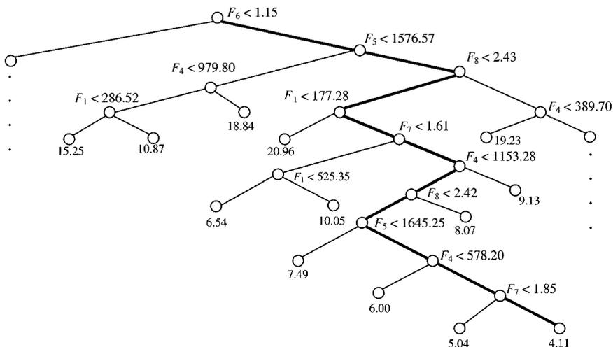
Figure 6. Part of the Classification Tree for the Fixture Layout Design.
