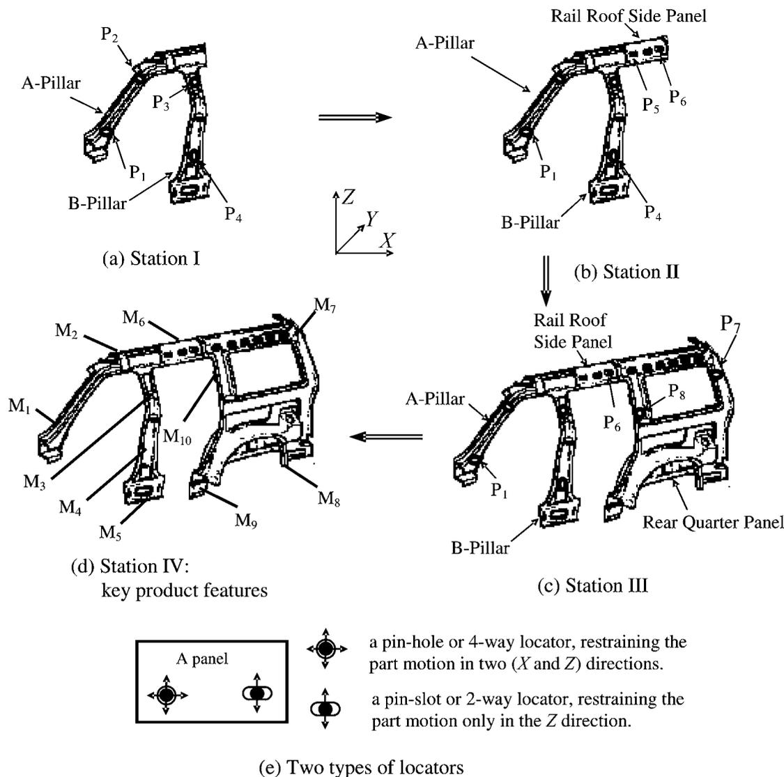
Figure 1. Assembly Process of an SUV Side Frame.
