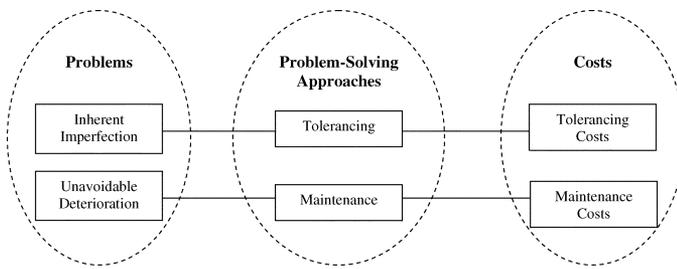
Fig. 1. Methodologies of improving manufacturing systems' performance.
