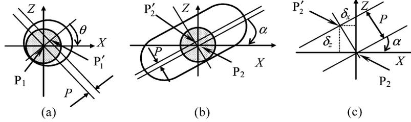
Fig. 9. Clearance-induced deviation.
