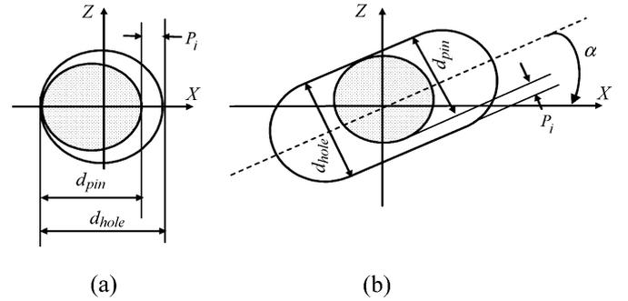
Fig. 5. Diagram of pin-hole locating pairs. (a) 4-way pin-hole; (b) 2-way pin-hole.
