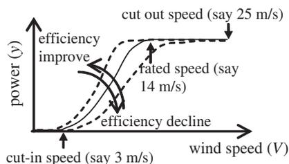
**Figure 1.** An example of a power curve and the associated power production efficiency.
