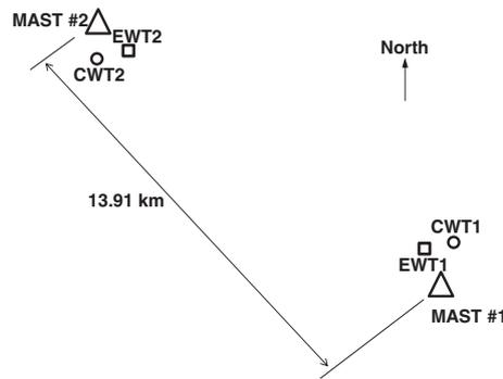
**Figure 5.** Wind farm layout. Triangles: meteorological masts; squares: experimental turbines that had an upgrade; circles: turbines in the control group that did not have the upgrade.
