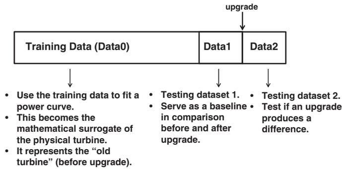
Figure 3. Data set partitions used in quantifying an upgrade.
