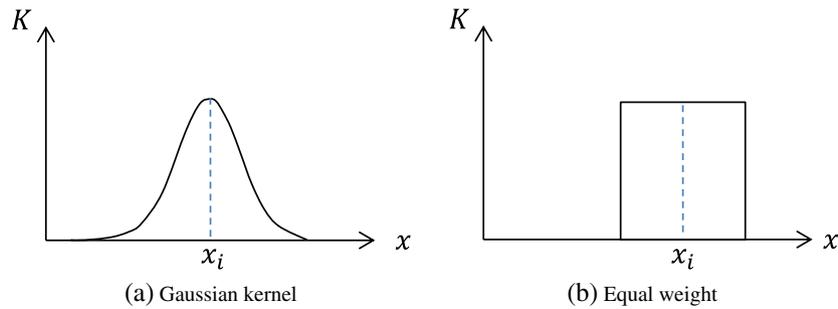
**Figure 2.** The kernel function in a kernel regression.
