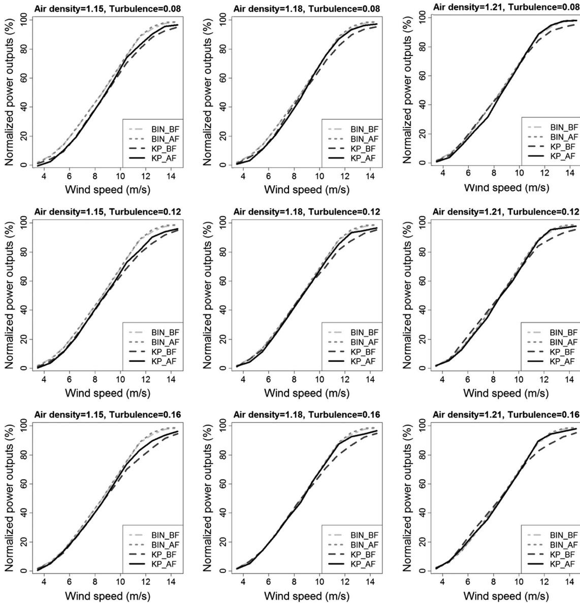
**Figure 8.** Power curves conditioned on air density and turbulence intensity and averaged across wind directions. The power outputs are normalized by the turbine’s rated power. BIN\_BF: binning method before upgrade; BIN\_AF: binning method after upgrade; KP\_BF: kernel plus method before upgrade; KP\_AF: kernel plus method after upgrade.
