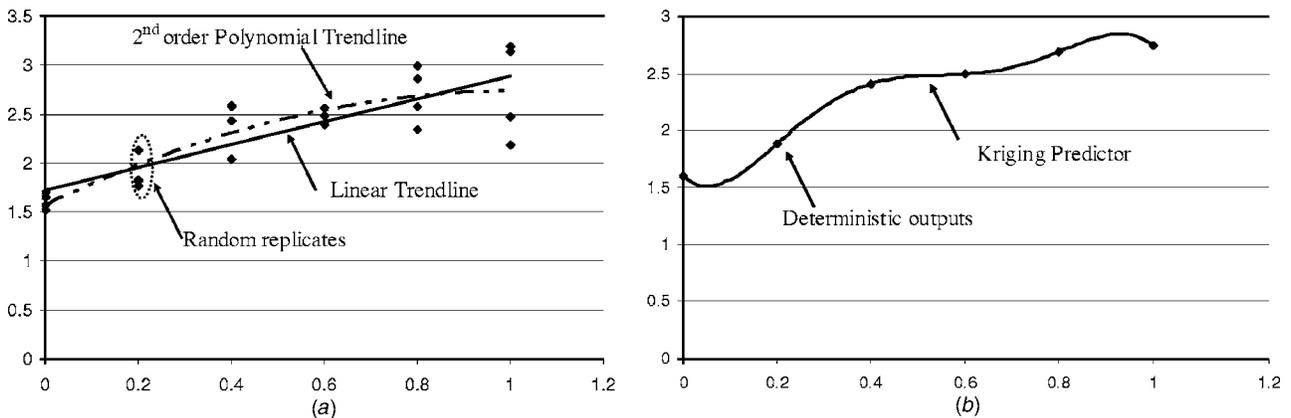
**Fig. 3 Difference between (a) physical and (b) computer experiments**
