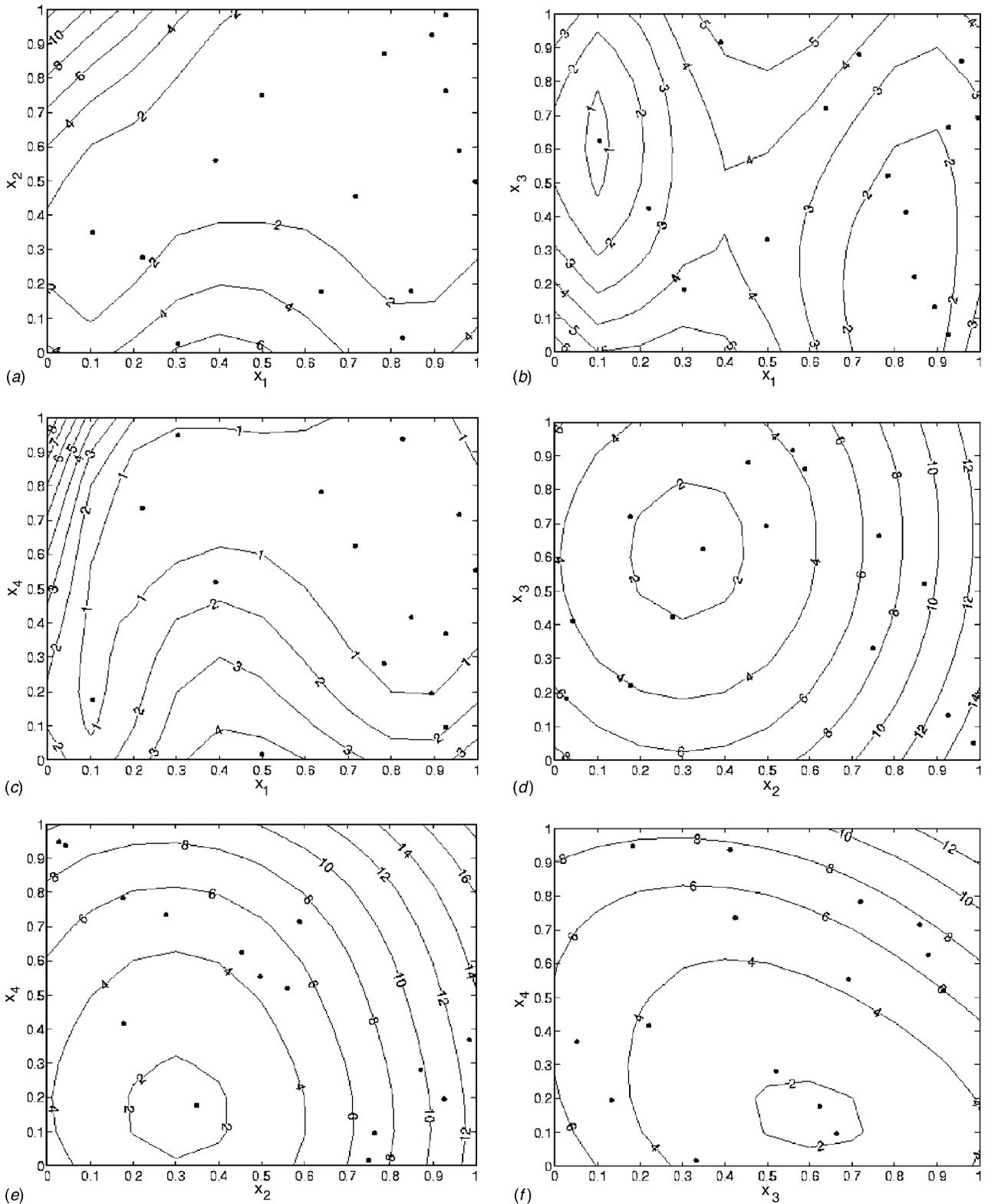
Fig. 8 MSE plots for pairwise design variables after the second stage
