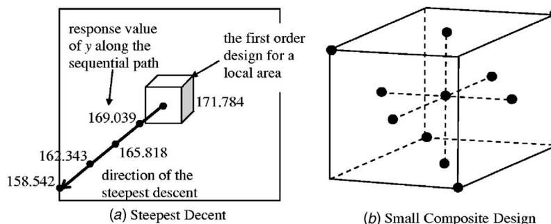
Fig. 11 Traditional response surface methodology for electronic packaging problem
