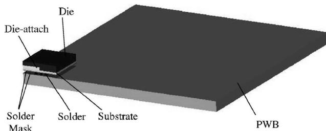
Fig. 2 The CSP-PWB model
