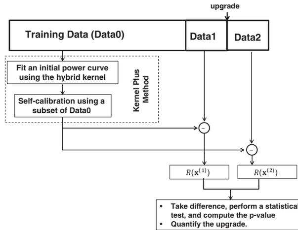
**Figure 4.** The procedure of quantifying a turbine upgrade using the kernel plus method.
