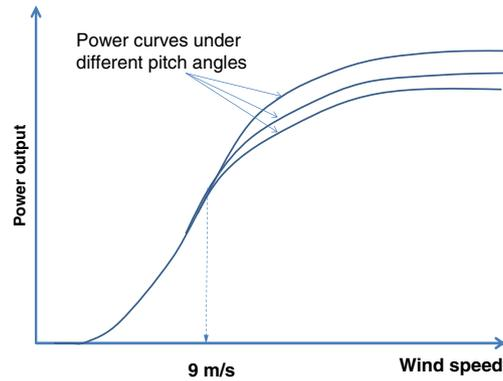
**Figure 6.** Illustration of power output results based on different pitch angles. This is a simplified adaptation from a figure in Wang *et al.*<sup>17</sup> The original work simulated three attack angles,  $5.5^\circ$ ,  $6.0^\circ$  and  $6.5^\circ$ , under the same designed tip speed ratio of 7 and designed wind speed of  $8.0 \text{ m s}^{-1}$ .
