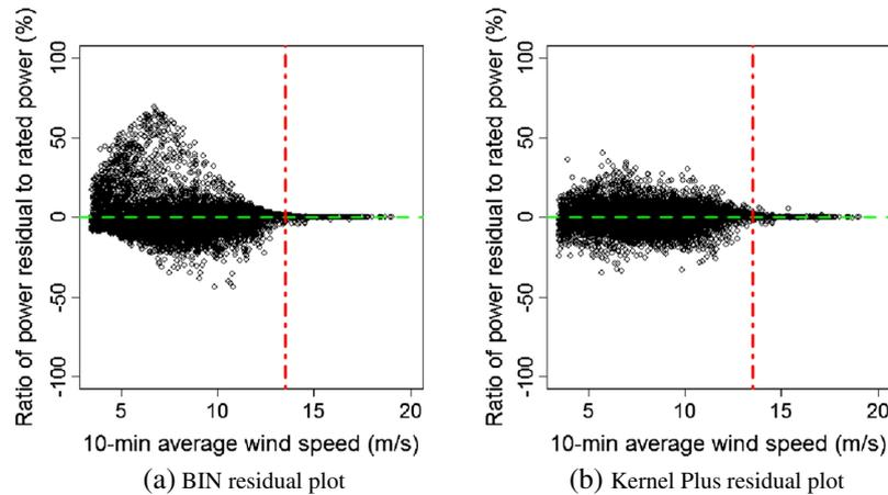
**Figure 7.** Residual plots after the binning method (left panel) or the kernel plus method (right panel) is applied. The vertical dashed line indicates the rated wind speed.**Table IV.** Comparing the kernel plus and binning methods on their ability to quantify a turbine's upgrade.
