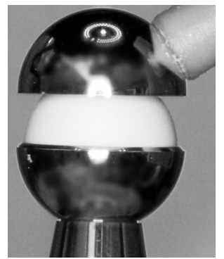
Lasers generate X-ray heat, causing the outer capsule to implode into the inner shell containing the deuterium and tritium mix. The resulting shock compresses the inner shell to generate the fusion reaction needed for energy-producing ignition.
